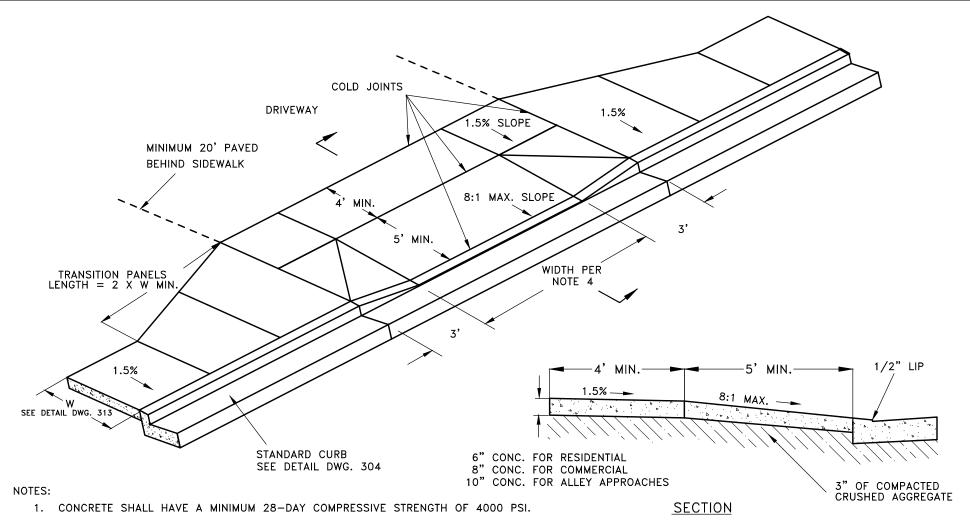
2. CURB AND GUTTER SHALL BE CONSTRUCTED INDEPENDENTLY, AND SEPARATED BY A COLD JOINT, FROM ALL ADJACENT CONCRETE CONSTRUCTION; INCLUDING SIDEWALKS AND DRIVEWAY RAMPS.
